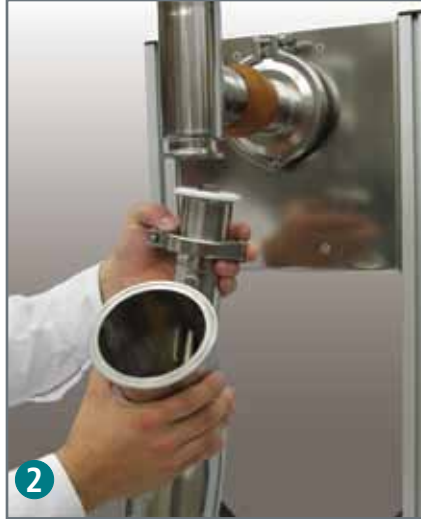
2 After clamp-release, the feed unit is easily removed.
