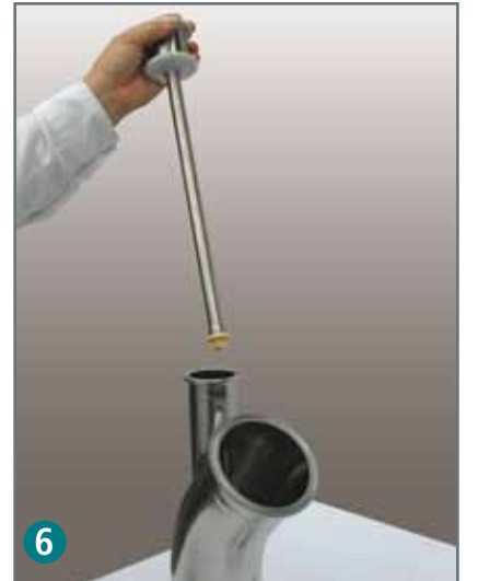
6 The drive shaft is easily removed.
