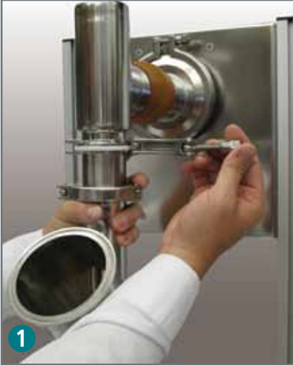
1 A sanitary quick release clamp allows you to disconnect the feed unit.
