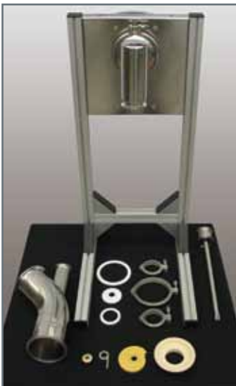
4 The bottom plate and ceramic feed disc are easily removed for cleaning and maintenance.
