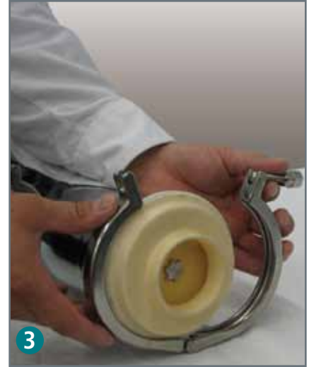
3 Place the feed unit on a flat surface where the clamp at the base of the feeder can be released.
