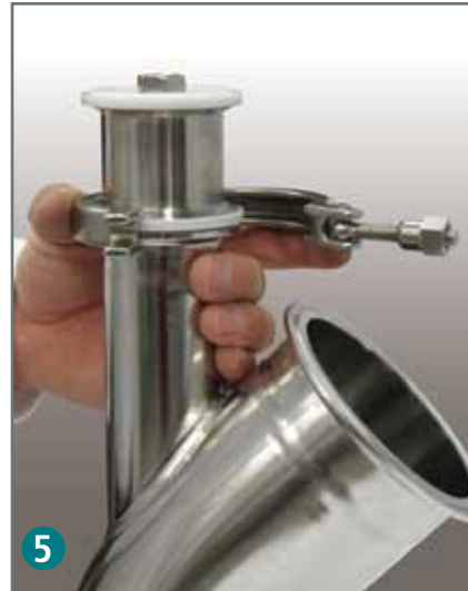
5 Disconnect the sanitary quick release clamp for drive shaft access.
