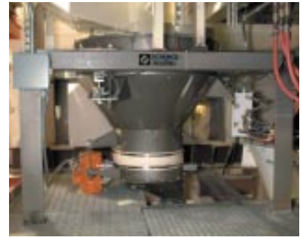
A vibratory feeder attached to the hopper's bottom induces material discharge.
