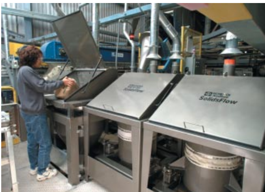
An operator manually adds material to the bag dump station, maintaining the material level in the hopper.
