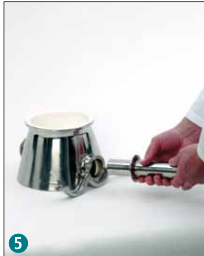
5 Nozzle slides out, allowing disposable hopper to be removed.
