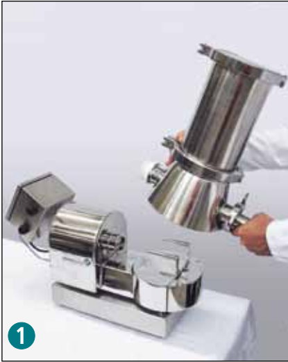
1 A single sanitary quick release clamp removes all product contact components.
