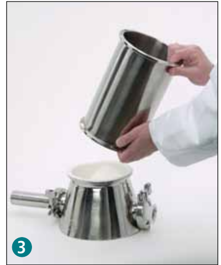
3 After releasing clamp the extension hopper is easily removed.
