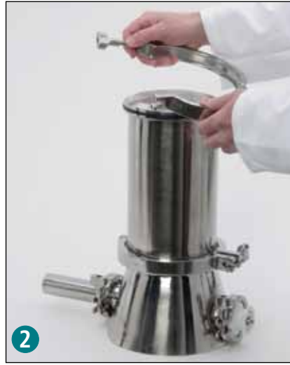
2 Cover is removed by disconnecting clamp.
