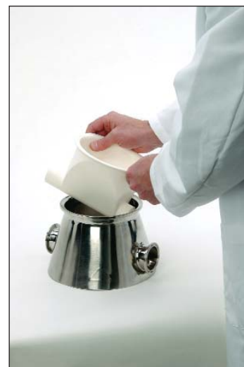
Figure 1: EPDM flexible hopper is disposable and reduces cleaning time.
